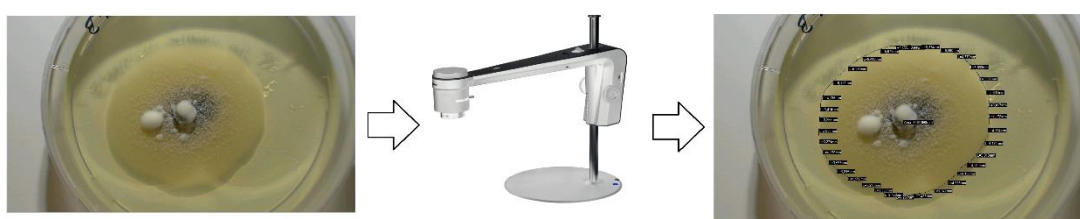
Figure 5: Illustration showing an example of the method for assessing colony radial area of Verticillium dahliae isolates using Tagarno. The petri dish was placed on the Tagarno. The digital microscope acquired a picture which was transfer to the software of the instrument on the computer. Measurement was made by manually rounded, with lines, the desirable area (colony radial area). After rounded the desirable area, result was presented in the middle in respective units, in this case mm 2 .
